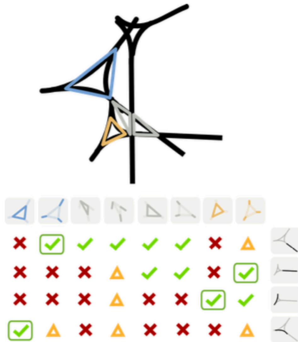
Figure 2. A simplified visual representation of the score matrix used for optimally assigning strokes to wedges. False positive candidate wedges are gray triangles. True positive candidate wedges are orange and blue. The green check mark signifies a match with high score, the orange triangle a match with low score and the red cross a match that is not allowed.
